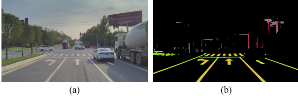
Fig. 3. Image segmentation. (a) is the raw image captured by front-view camera. (b) is the semantic segmentation result. The orange and gray pixels indicate ground markers and poles, respectively. Green pixels highlight the outline of the ground markers and red pixels indicate the fitted straight lines of the poles. Note that short poles are discarded to avoid bringing in noise.
