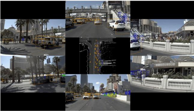
Fig. 5. Examples of nuPlan sensor data. We can see the lidar data and map in the center and 6 camera views around it. All views show the highly accurate autolabeling annotations.
