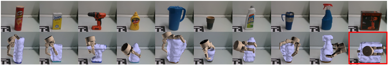
Fig. 7: Example grasps proposed by Multi-FinGAN on real objects. The upper row shows the unsegmented input image and the bottom rows shows some grasps on the shape-completed object. The grasp shown in the red box failed as it was in collision with the object.
