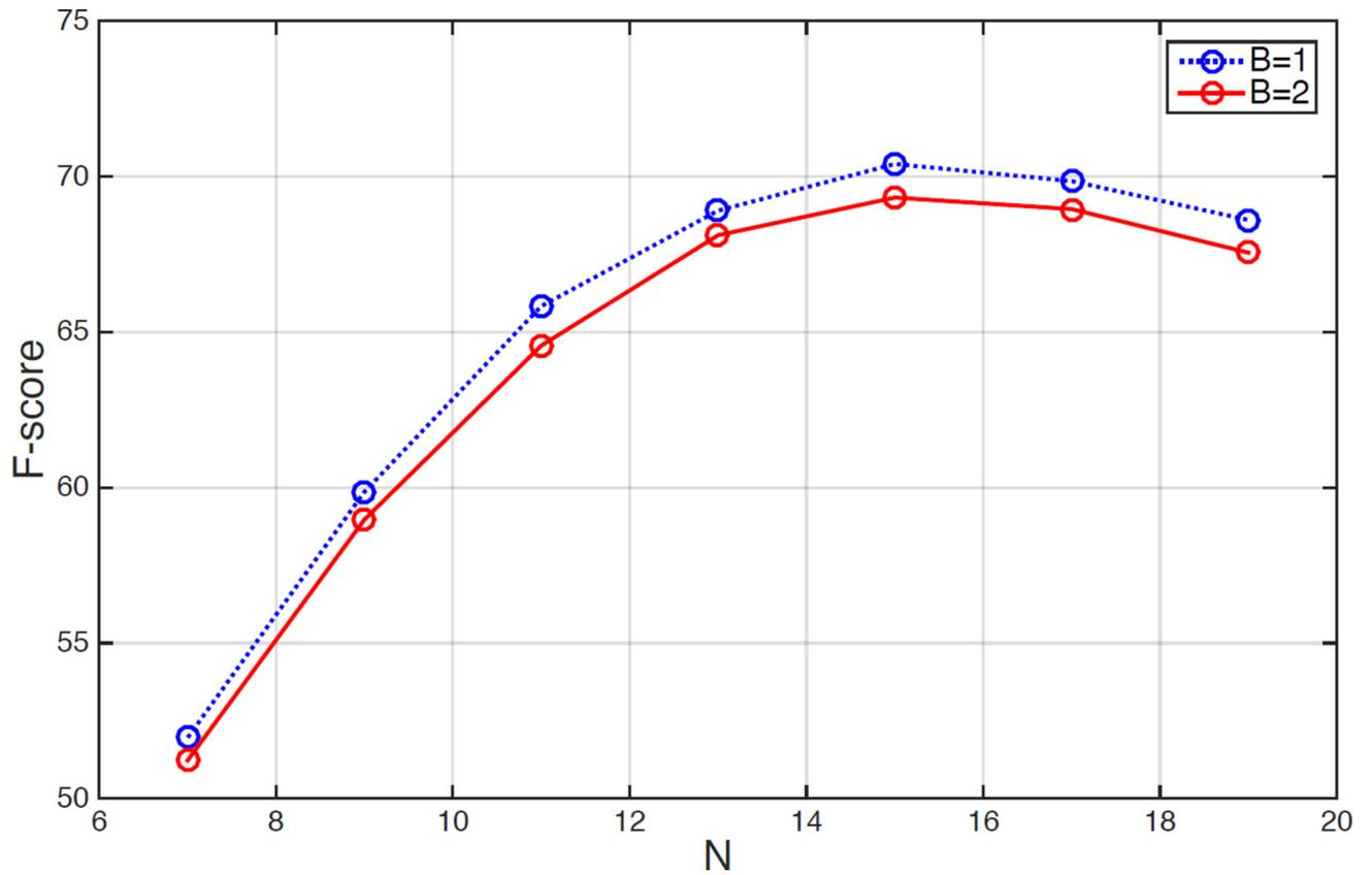
**Figure 6.** The F-score of ours system on the ICDAR 2015 incidental dataset as a function of the parameters  $N$  (which determines the number of cells in grid considered by WordDetNet) and  $B$  (the number of boxes generated per cell).
