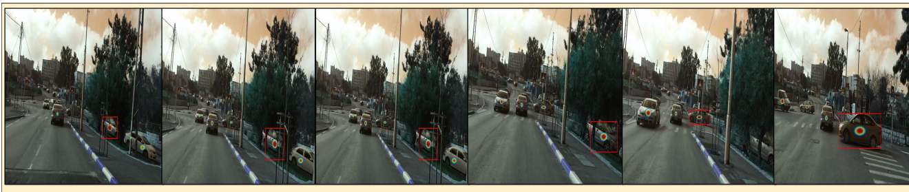
Figure 8: Explainability via Attention. A sequence of frames, with superimposed heat-map as calculated using the spatial attention weight in each frame. The object with the highest attention score is shown in the red bounding box, and the heat-maps of the other objects describe their weights with respect to the red bounding box.
