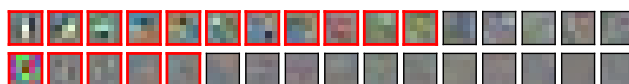
Figure 1. The low-rank basis of filters in the first layer of the convolutional neural network [16] on CIFAR-10. The low-rank basis is formed by the most significant principal filters that are obtained by PCA. Top: the low-rank basis of the original network. Bottom: the low-rank basis of the same network after applying Force Regularization. The number of red boxes indicates the required rank to reconstruct the original filters with \leq 20\% error.
