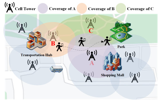
Fig. 1. An example of cell tower distribution in a region. Purple, orange and green ellipses indicate the coverage of the cell tower A, B and C. Blue ellipses means the coverage of other cell towers. The coverage areas of different cell towers are partially overlapped, so users can switch between cell towers and still maintain the connection.
