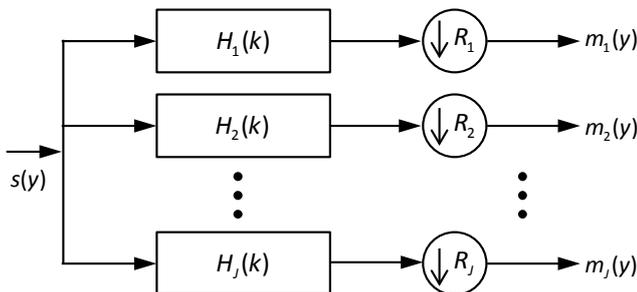
Fig. 1. Multichannel sampling.
