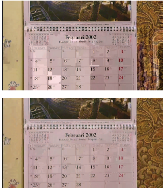
Fig. 3. Frame 160 of Mobile Calendar sequences without (top) and with (bottom) continuous drift correction. PSNR improves from 20.42 dB to 25.30 dB.
