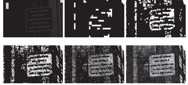
Fig. 4. Homogeneous block selection for the image in Fig. 2 using various block sizes, k = 64, 32, 16, 8, 4, 2 (left to right and top to bottom). Homogeneous regions are shown as white areas.
