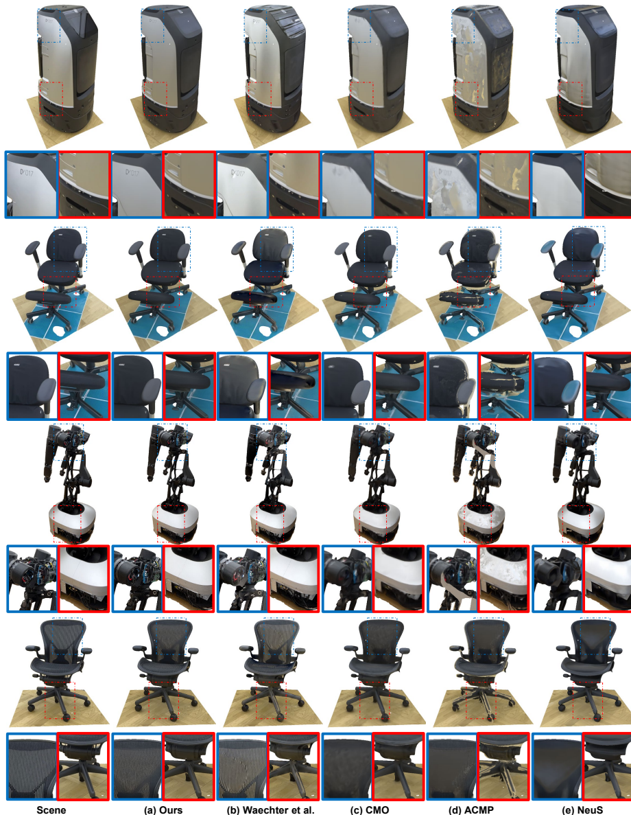
Figure 7. Qualitative comparison between (a) Ours, (b) Waechter et al. [53], (c) CMO [69], (d) ACMP [62], and (e) NeuS [55]. Compared to textured mesh (3-6 columns) obtained from different algorithms, the result of our method is perceptually closer to the original scene. Additional qualitative results are added in the supplementary material due to the limited space.
