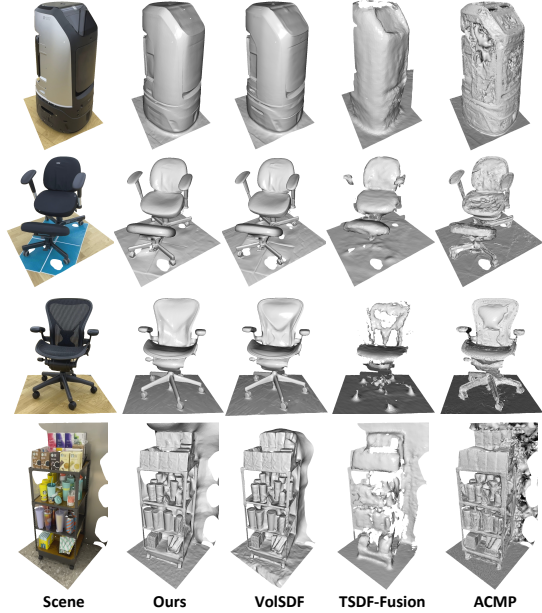
Figure 6. Reconstruction of our method, VolSDF [63], TSDF-Fusion [23], and a mesh from point clouds of ACMP [62] processed with screened Poisson surface reconstruction [27]. Note that the neural surface reconstruction is more perceptually convincing in the ARKit-video dataset.
