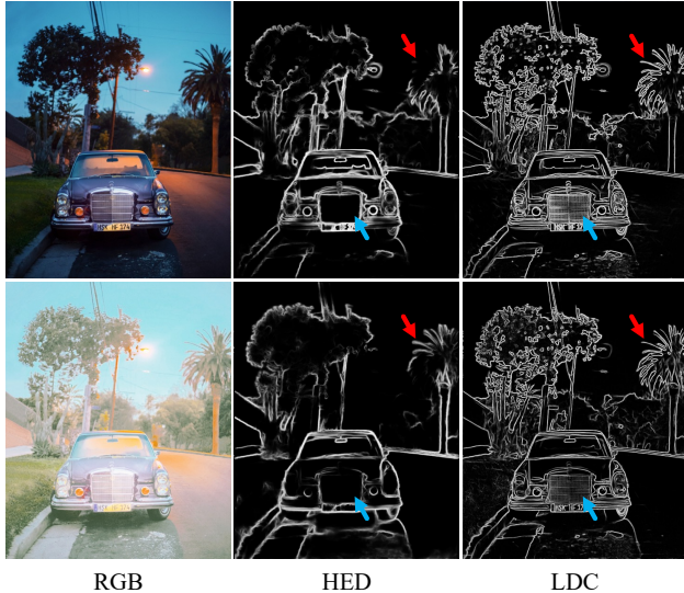
Figure 15. Predicted Edges for Content Similarity Calculation. For a more precise quantitative evaluation of content similarity, we replace HED [74] (used by prior works [1, 50, 77]) with LDC [66]. LDC can provide finer (see blue arrows) and more accurate edges (see red arrows) than HED.
