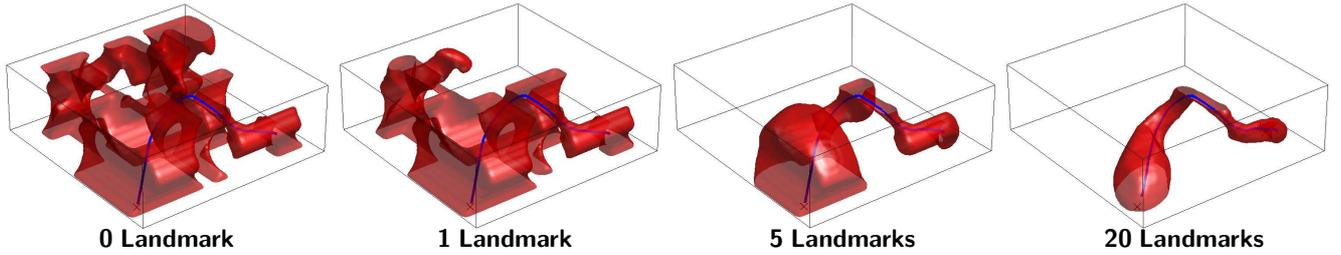
Figure 9. Explored area for constrained path planning.
