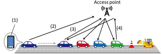
Fig. 3. Demonstration scenario. (1) Obtain own location and orientation (2) Join the multicast group (3) Request the description with multicast (4) Respond to the request
