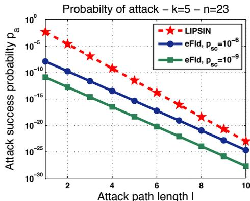
Figure 1: Attack probability,  $p_a$ , using proposed eFID or LIPSIN over different path-lengths. eFID:  $m = 256$ ,  $|h| = 64$ . LIPSIN:  $m = 320$ . Bloom filter has 23 LIDs with  $k = 5$ .
