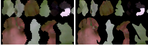
Figure 3: Close-up of the image texture of a mesh, generated with the same texture atlas but different resolutions. (Left: 80 \times 50 , Right: 320 \times 200 ).
