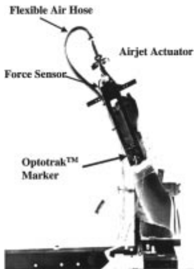
Fig. 6. The airjet actuator attached to a subject's wrist.
