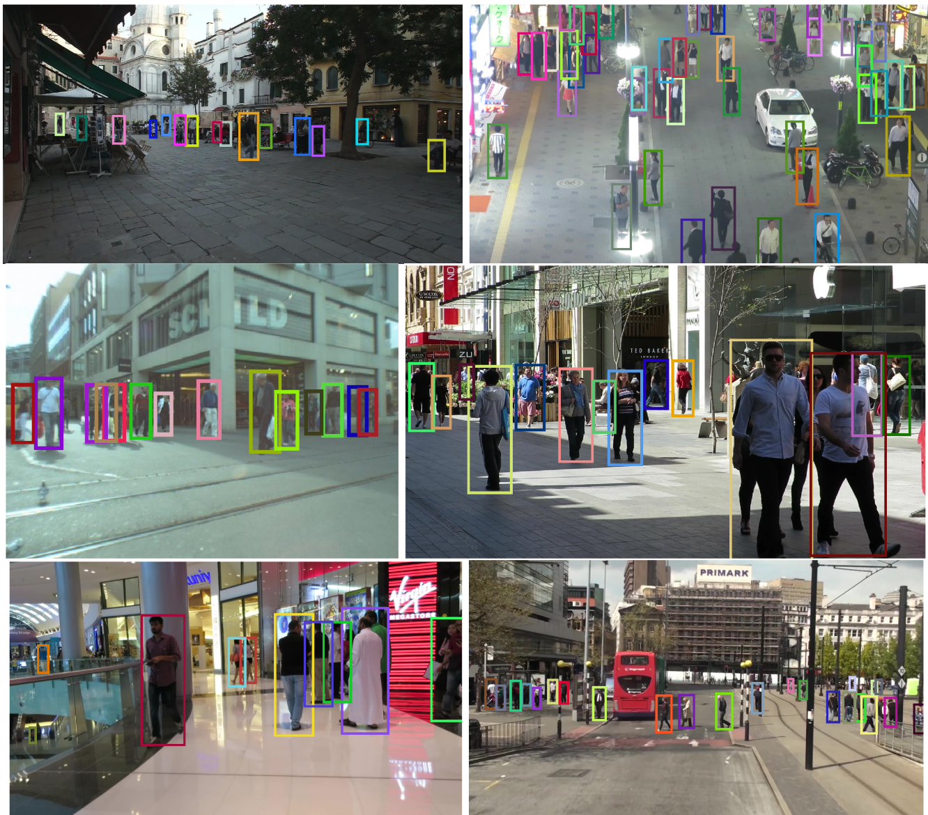
Fig. 4: Sample results on several sequences of MOT17 data sets using SDP detector; bounding boxes represent the tracking results with their color-coded identities. From left to right: MOT17-01-SDP and MOT17-03-SDP (top row), MOT17-06-SDP and MOT17-08-SDP (middle row), and MOT17-12-SDP and MOT17-14-SDP (bottom row). The videos of tracking results are available on the MOT Challenge website https://motchallenge.net/ .
