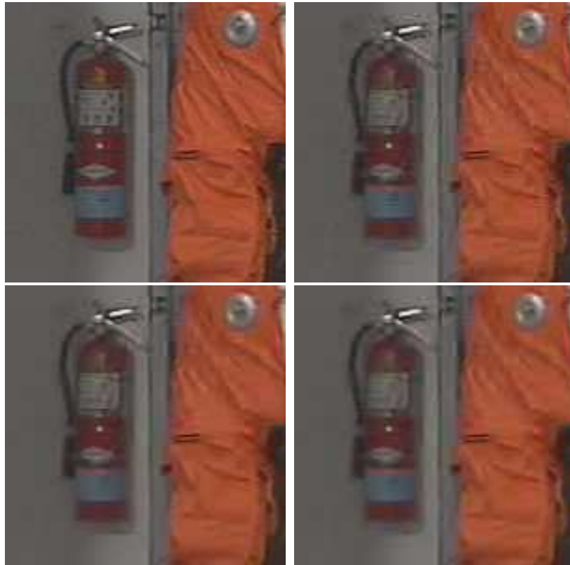
Figure 6: Part of P-frame from test sequence Crew. Upper left) Original. Upper right) MPEG-2 decoded (36.02 dB). Lower left) Deblocking and deringing using estimated Q_S values ( EQ_S ) (36.38 dB). Lower right) Embedded deblocking using code stream Q_S values (36.45 dB).
