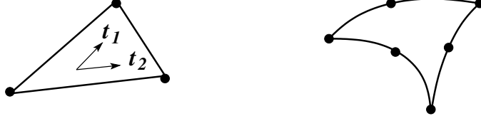
Figure 3: In the simplest geometric model, the surface of the scatterer \partial D_1 is approximated by a collection of flat triangles, defined by the locations of its three vertices in \mathbb{R}^3 . On each triangle, there are two linearly independent tangent directions \mathbf{t}_1 and \mathbf{t}_2 . The unknown electric and magnetic currents \mathbf{J} and \mathbf{K} on each triangle are defined by j_1\mathbf{t}_1 + j_2\mathbf{t}_2 and k_1\mathbf{t}_1 + k_2\mathbf{t}_2 , respectively, and the electromagnetic fields are evaluated at the triangle centroids. For higher order accuracy, each quadratic surface patch is specified by six nodes: the three triangle vertices and three additional points, one on each curved triangle side. Three “support nodes” \mathbf{x}^1, \mathbf{x}^2, \mathbf{x}^3 are then selected in the interior of each patch. Our representation for \mathbf{J} and \mathbf{K} at each support node \mathbf{x}^i is of the form j_1^i\mathbf{t}_1^i + j_2^i\mathbf{t}_2^i and k_1^i\mathbf{t}_1^i + k_2^i\mathbf{t}_2^i , where \mathbf{t}_1^i, \mathbf{t}_2^i are linearly independent tangent vectors at \mathbf{x}^i . The support nodes are also the points where we evaluate the electromagnetic fields and impose interface conditions.
