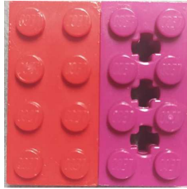
Figure 9 Red (left) and spoiled red (right) bricks.
