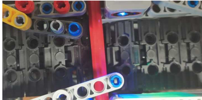
Figure 17 Distance limiter parts and the colour sensor.
