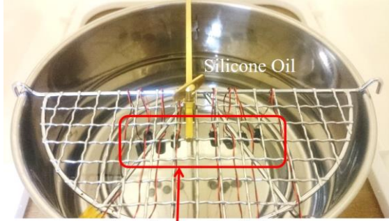
Fig.2 Experimental setup of accelerated ageing test with an oil bus.
