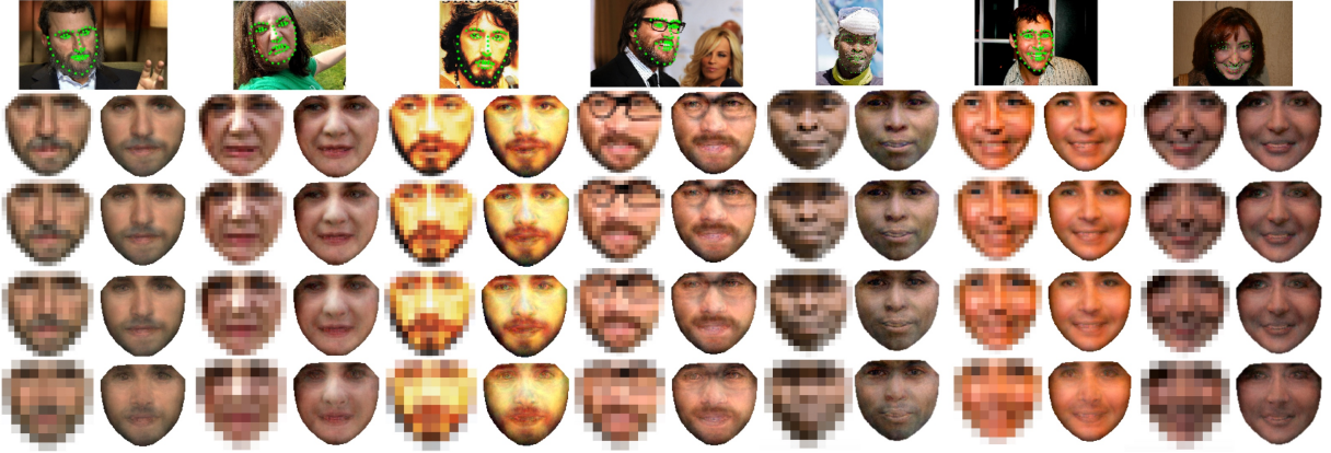
Fig. 6 Facial image super-resolution reconstruction at different scales of down-sampling. The 1st row: original image, the 2nd row to the 5th row: down-scaled images with factors of 4, 6, 8, 12 (left) and reconstructed facial images using DAMs (right).
