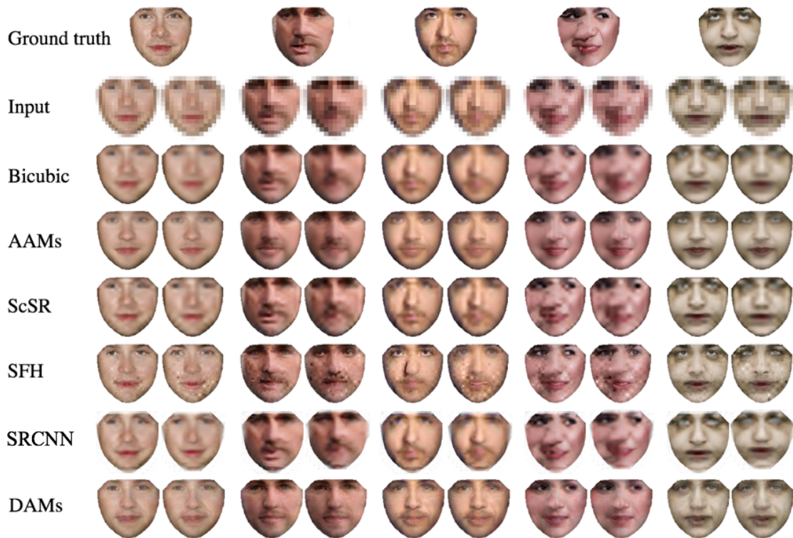
Fig. 8 Comparisons of different facial image super-resolution methods. The 1st row: ground truth faces. The 2nd row: down-scaled images with factors of 6 (left) and 8 (right). From the 3rd row to the 8th row: reconstructed faces using bicubic, PCA-based AAMs, ScSR (Yang et al, 2010), SFH (Yang et al, 2013), SRCNN (Dong et al, 2014) and DAMs, respectively.
