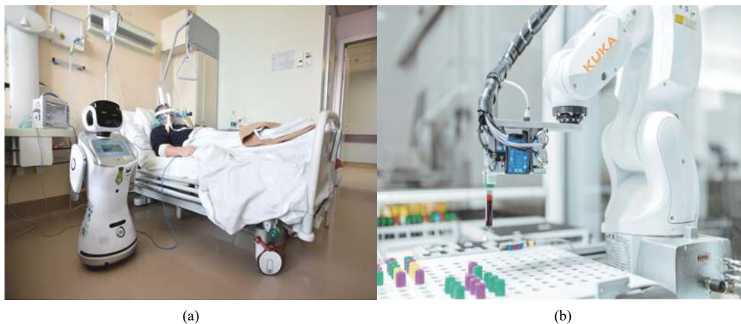
Fig. 2 Robotics in telemedicine: (a) Remote observation of patient using a robot; (b) Blood sample handling robots.
