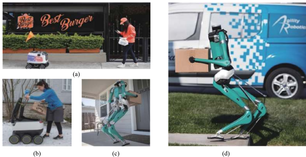
Fig. 7 Robotics in material delivery: (a) Food delivery via robot without any human contact [47] ; (b) Starship technologies autonomous food delivery robot [48, 49] ; (c) and (d) Ford and Agility Robotics autonomous legged robot [50] .
