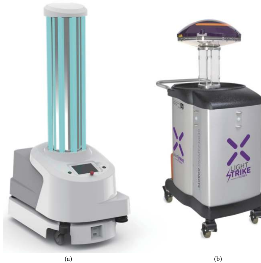
Fig. 3 Sanitizing robot: (a) UVC disinfection robot by UVD Robotics; (b) LightStrike germ zapping robot with pulsed Xenon UVC
