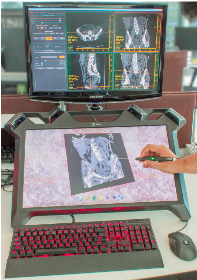
Fig. 1 An image of the hybrid interface showing the 2D display at the top , followed by the zSpace display at the bottom . The image also shows mouse, keyboard, and the 3D stylus input
