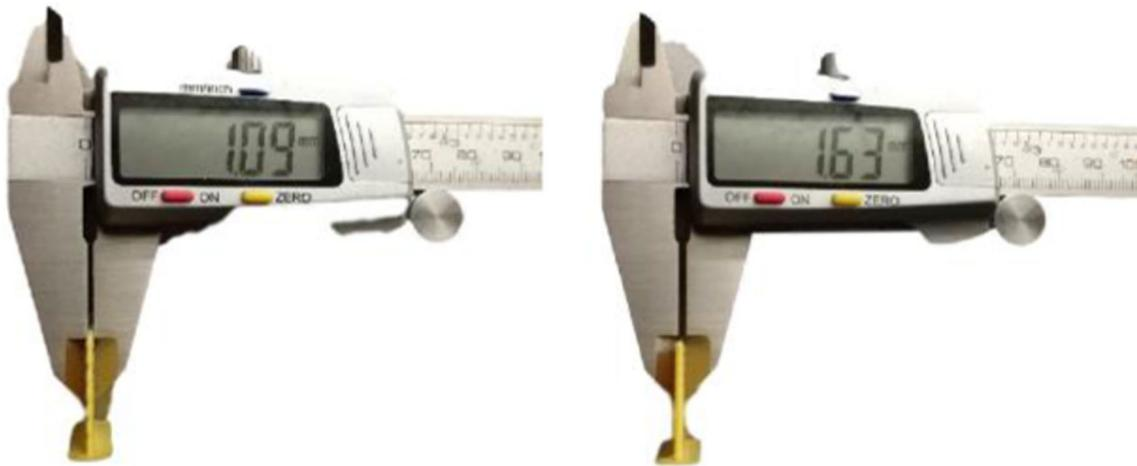
Fig. 2 Error due to filament diameter variations
