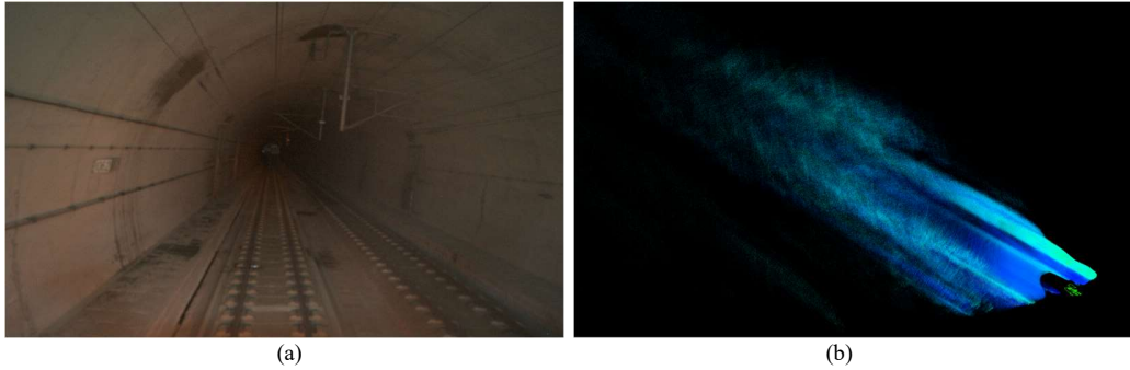
Figure 27. Examples of LiDAR SLAM failure in tunnels. (a) is the image view of a high-speed railway tunnel. (b) presents the real-time mapping and odometry output of LOAM. It is seen the mapping is blurred with the odometry output ‘stopped’ due to degeneration.
