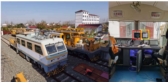
Figure 36. The exterior and interior of the autonomous driving maintenance rail vehicle. The screen in the red rectangle shows the real-time positioning result as well as the ATCS based warning information. The screen in the yellow rectangle shows the train automatic control information, such as pressure, brake, and acceleration.
