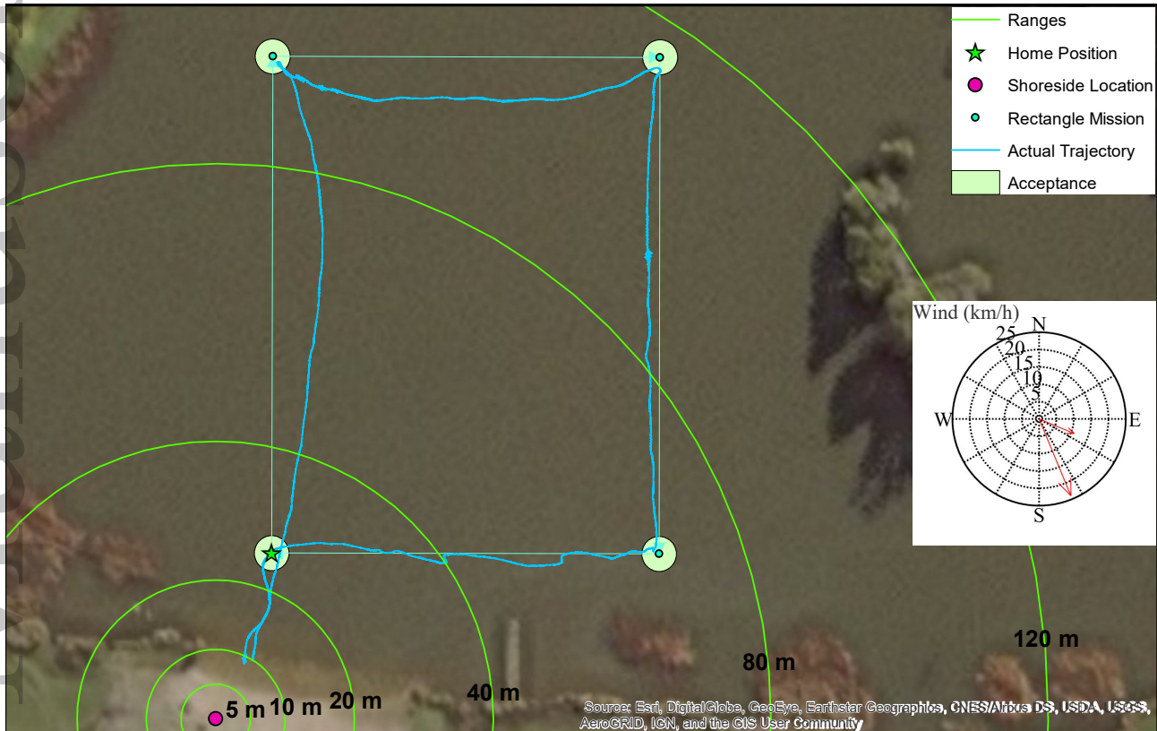
Figure 13: One of the rectangle missions performed by the ASV. Strong and intermittent North-Westerly gusts blew the vehicle sideways from the expected trajectory, leading to trajectories with cross-track errors that are sometimes large and sometimes small. The autopilot controller does not control motion in the sway direction, leading to arcs in the achieved trajectory.
