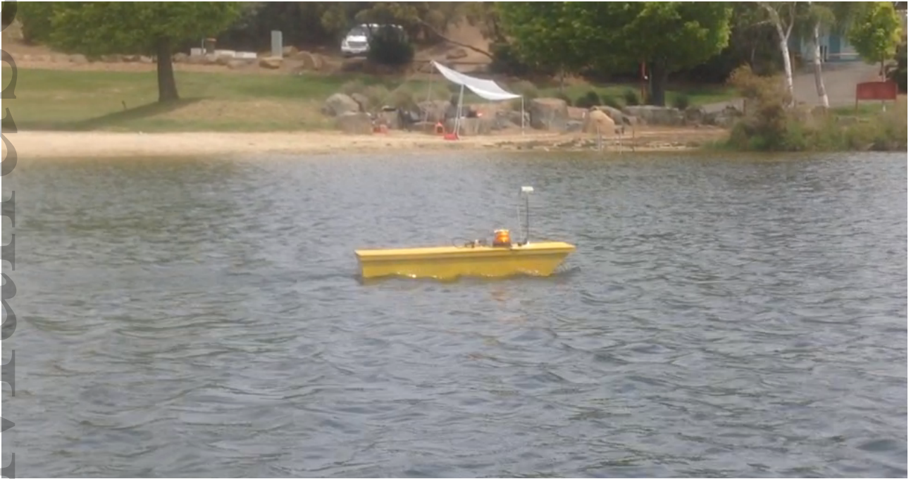
Figure 12: The ASV underway on a waypoint following task in Lake Waverley. Shoreside system setup in background.
