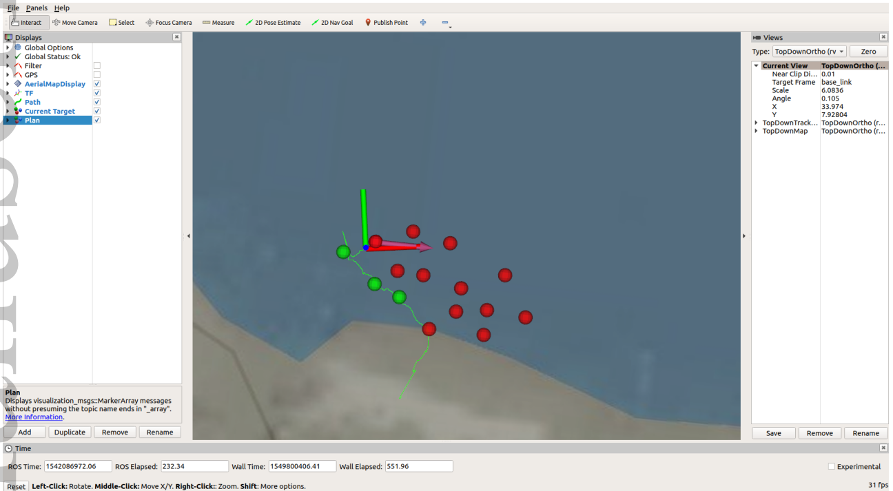
Figure 3: Screenshot from the HMI component of the shoreside system. The vehicle's position and orientation is provided by the red/green/blue axis, incomplete waypoints are shown as red spherical markers, completed tasks are shown in green. The selected waypoint for completion is shown with a red marker and fuchsia arrow.
