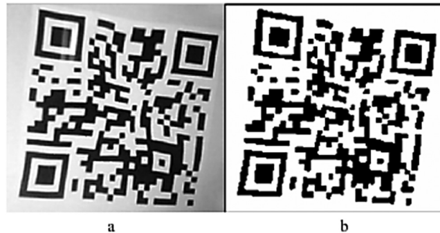
Figure 10: Binarization effect diagram: (a) Before binarization and (b) After binarization.
