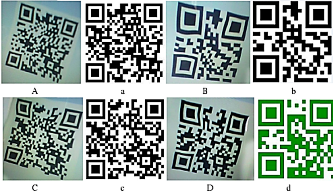
Figure 4: Sample picture collection indicated by capital (A–D) and the corresponding QR codes indicated by small (a–d).
