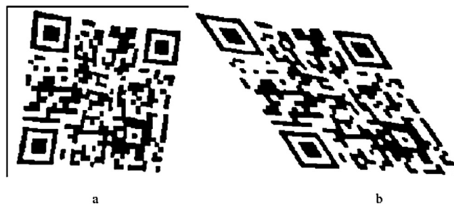
Figure 11: The result of distortion correction processing: (a) Before distortion correction and (b) After applying distortion correction processing.
