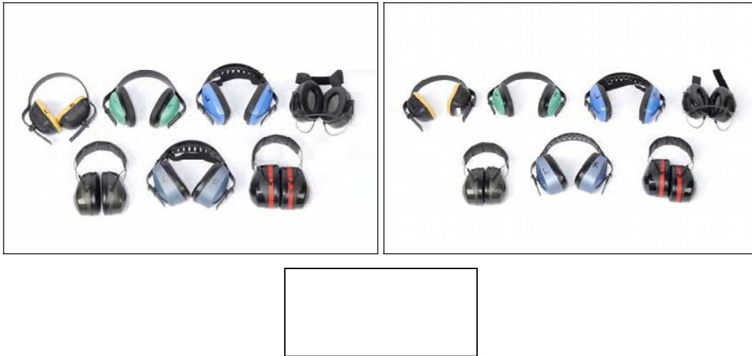
Figure 4 New (left) and artificially aged earmuffs (right)
