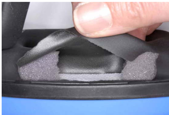
Figure 5 Break to cup seal simulating seal damage
