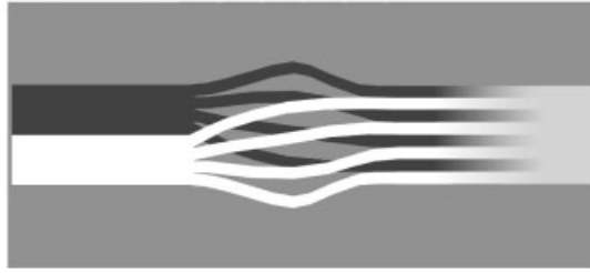
Fig. 4.11 Principle of a laminating mixer – the main idea is to minimize the necessary diffusion lengths.
