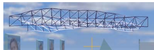
The wind starts the bridge oscillating
