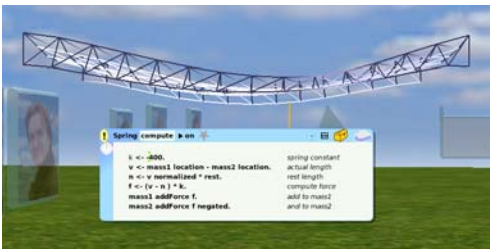
Making the bridge structure springy
