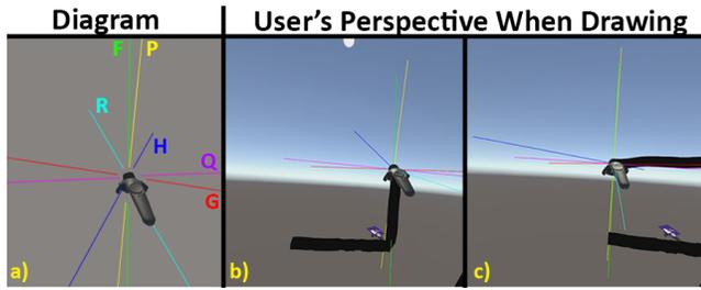
**Figure 6: SG-crosshair always follows the controller orientation and position.**
