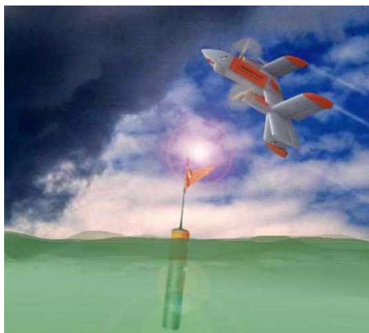
Figure 1: A Typical UAV Mission: Deployment and Monitoring of Acoustic Sensors
