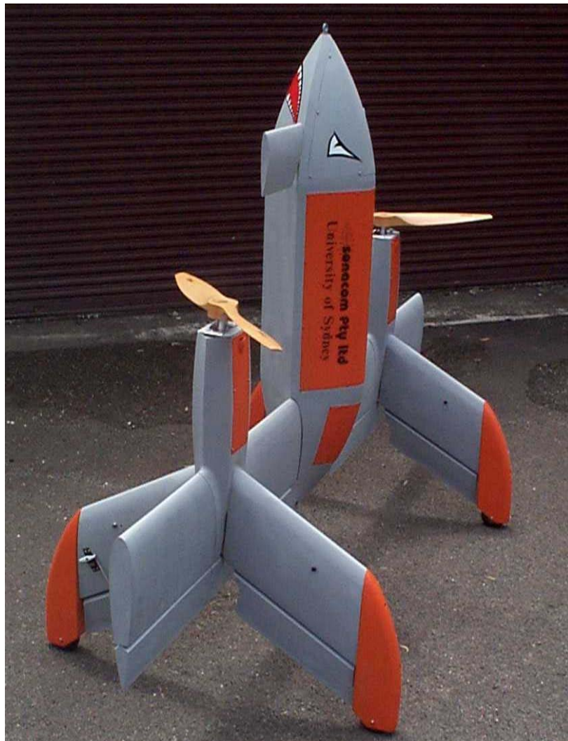
Figure 3: Completed T-Wing Technology Demonstrator Vehicle, (Electric Powered Configuration).
