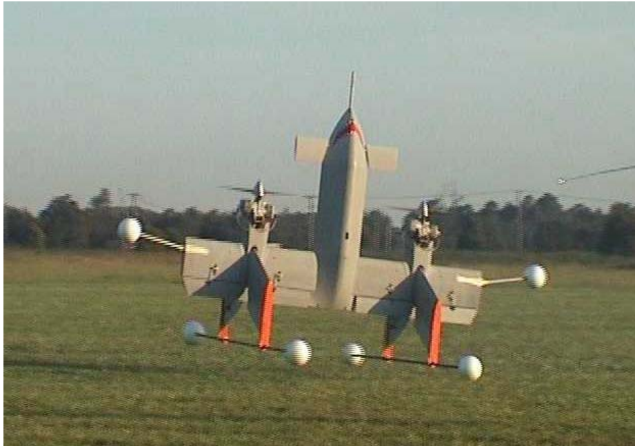
Figure 4: First Free Flight of T-Wing Technology Demonstrator Vehicle under Manual Control. (Note "training" undercarriage").
