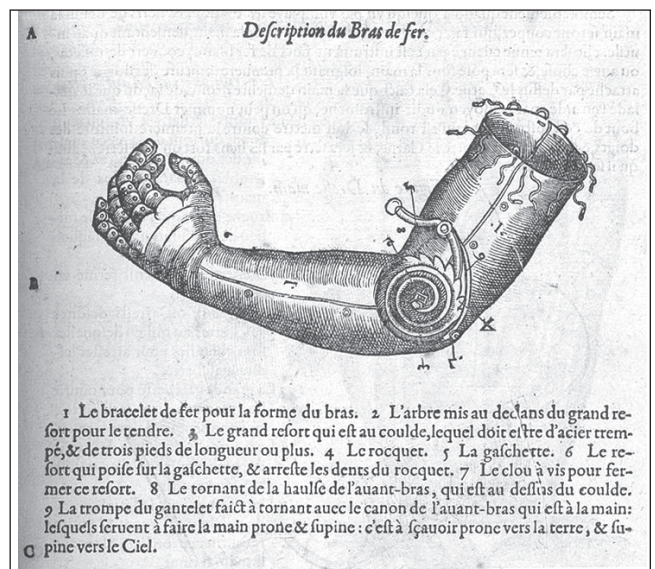
Figure 4) Description of Paré's iron arm design for an above-elbow amputee. A lever-sprocket mechanism controls elbow flexion and extension. Image retrieved from US National Library of Medicine < www.nlm.nih.gov/exhibition/historicalanatomies/home.html >
