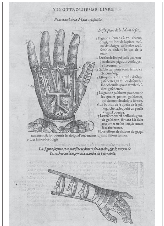
Figure 3) Ambroise Paré's illustration of the 'Le Petit Lorrain' prosthetic hand published in 1575 in his book Les oeuvres d'Ambroise Paré (The Works of Ambroise Paré). Although the wrist is immobile, the fingers are held in extension by four springs fixed in the palm. The fingers may be brought into flexion and are kept in position by sprockets controlled by metal levers, thereby allowing a reliable grip on objects. The hand is connected to the forearm stump with two metal bars and leather straps. Image retrieved from US National Library of Medicine < www.nlm.nih.gov/exhibition/historicalanatomies/home.html >
